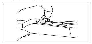
3. Pull the clip up from the blade connecting point, and pull the blade assembly down toward the windshield to remove it from the wiper arm.
